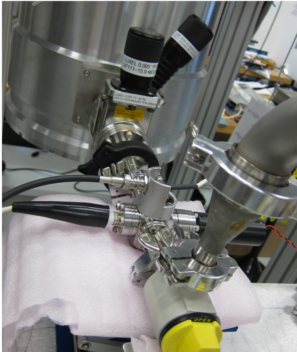
GSFC Modulated X-ray Source attached to lab dewar
