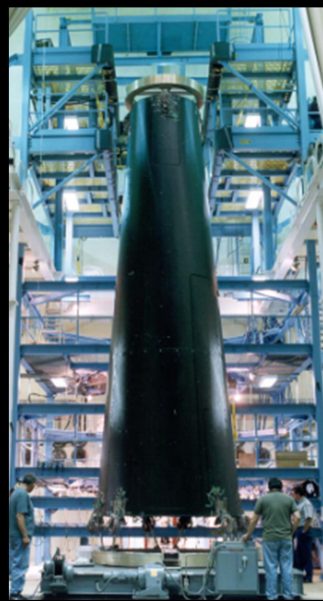
Completed OBA with blankets installed being prepared for HRMA integration at NGAS
