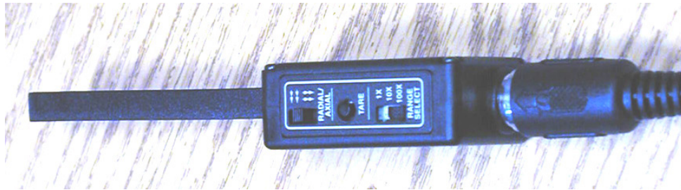
Figure 2 Magnetic field sensor , showing (from right to left) the range select switch, the tare button, and the radial/axial switch, which is set to radial.
