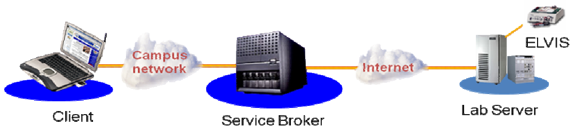
Figure 2-1: The iLab Shared Architecture showing the various components of the architecture and where the ELVIS is plugged into the architecture [13].
