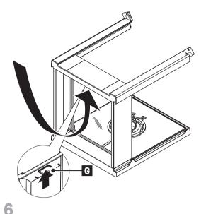
Push the lock button (G) to release the rear glass.
