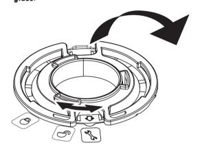
a) Turn the **draft shield lock** to the ""\" (Service) position.
