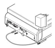
Connect the AC adapter to the connection socket on the back of your balance (see figure) and to the power line.
