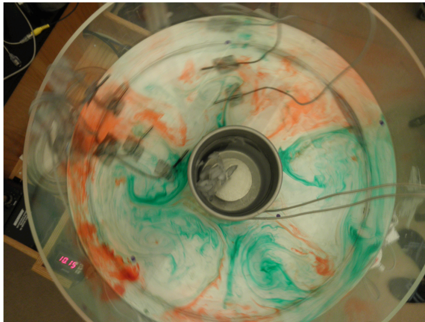
Fig. 1 An overhead view of the laboratory experiment. The red dye began at the edge of the tank, and the green dye began at the center.
