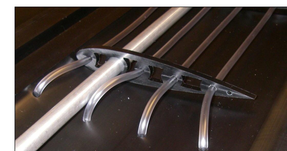
Above: NACA 0018 foil molded from solid urethane and instrumented with four commercial pressure sensors Left: Pressure transmission tubes molded within foil
