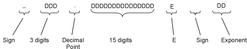
Figure 4-1 FORM4 (ASCII) Data-Transfer Character String
