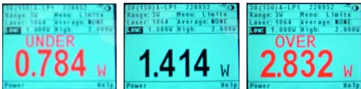
Figure 4.9 Limits Screens with limits set to 1W and 2W
