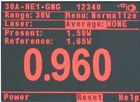
Figure 4.3 Thermopile Normalize Screen
