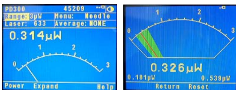
Figure 4.10 Needle Screens with a photodiode sensor
