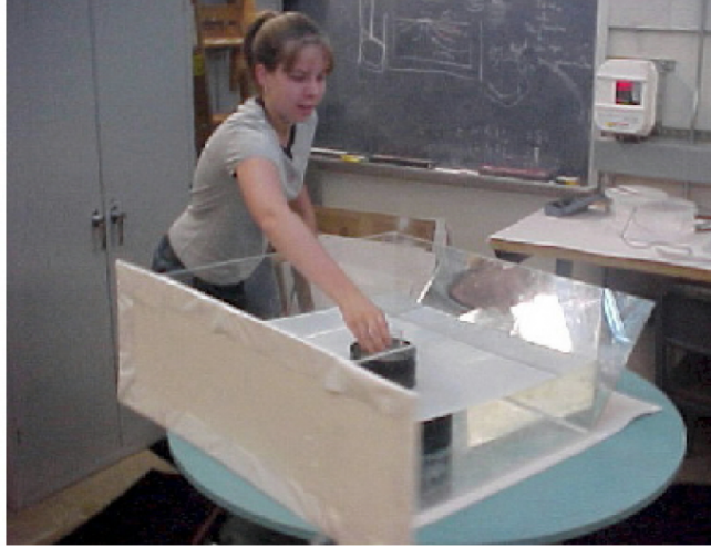
Figure 2: Setting up the rotating tank to create a front. By placing dense fluid (high salinity water) in the center of the rotating tank, we can create a dense cone surrounded by less dense water. This creates a density gradient capable of creating currents observable at the surface. These currents are analogous to jets high in the troposphere. Image from the Project 2 explanation by John Marshall and Lodovica Illari at http://www-paoc.mit.edu/12307/front/project2.pdf . (Illari and Marshall a)
