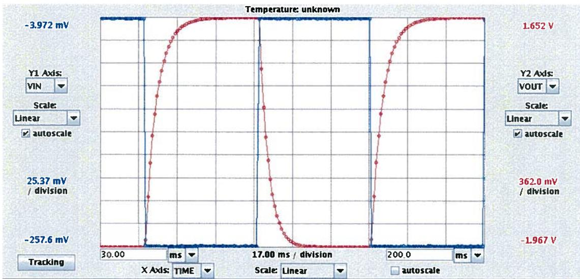
The time constant for both rising and falling output is  $\sim 5$  ms.
