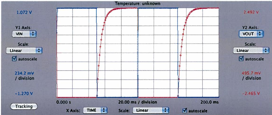
The rising and falling time constants can be found by finding the slope at the time when the output is rising and falling respectively.
