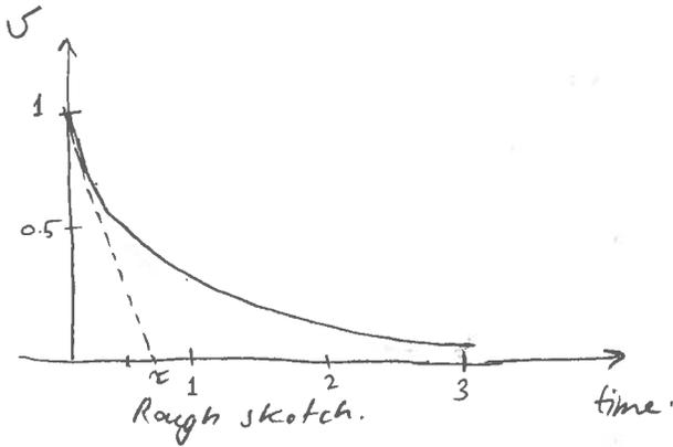
Network had been assembled for a long time. At  $t=0$  the current source turns off.
