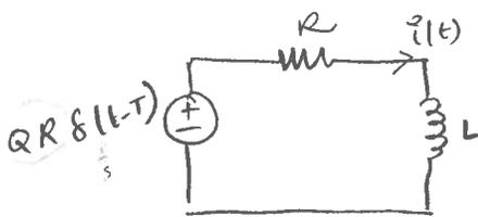
similar to that in part (a), the impulse voltage source results in a flux dump in the inductor causing the current to rise instantaneously
