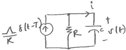
The impulse current @  $t=T$  results into a charge dump on the capacitor which causes the voltage across the capacitor to change instantaneously:
