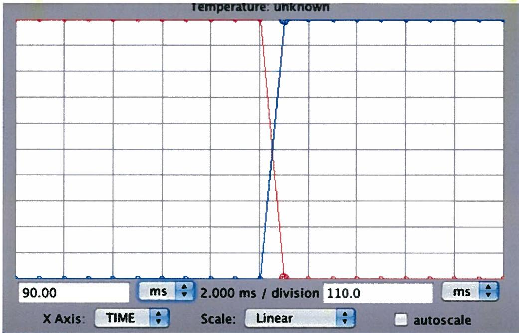
At falling edge of the output the time constant is really short as seen as a sharp fall in the output. From the above figure, it is seen that the time constant is much less than 1ms since the output falls from high to low in 1ms.
