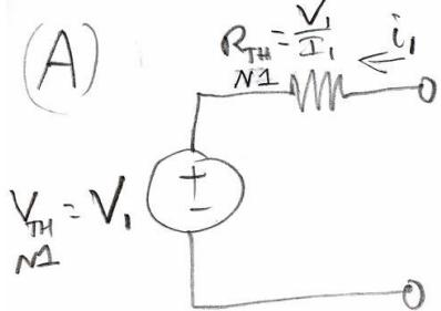
For N1:  $V_{TH} = V_{OC} = V_1$ ,
