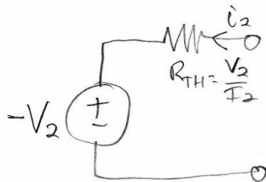
$$V_{TH} = V_{OC} = -V_2; \quad I_N = -I_{SC} = -I_2; \quad R_{TH} = \frac{V_{TH}}{I_N} = \frac{-V_2}{-I_2} = \frac{V_2}{I_2}$$
