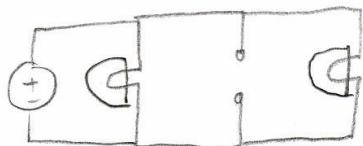
3<sup>rd</sup> Circuit) Brighter - the current and power, as  $P = I^2 R$ , increase as the same total current is now split between the 2 remaining bulbs.
