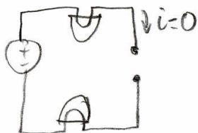
2<sup>nd</sup> Circuit) No Change - with all 3 bulbs in parallel, the voltage and power, as  $P = \frac{V^2}{R}$ , will remain constant on the 2 remaining bulbs
