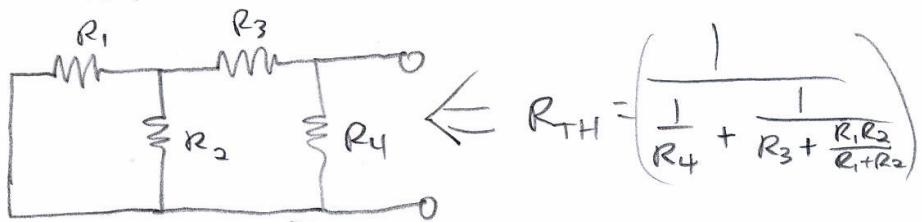
$R_4$  is in parallel with the series combination of  $R_3$  with the parallel combination of  $R_1$  and  $R_2$ .
