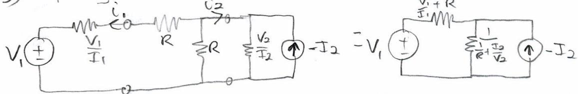
$$i_1 \text{ is still the total current out of } N1, \text{ using superposition and voltage and current dividers:}$$
