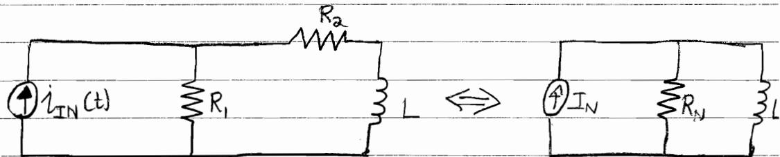
$$I_N = \frac{R_1}{R_1 + R_2} i_{in}(t) \quad R_N = R_1 + R_2$$
