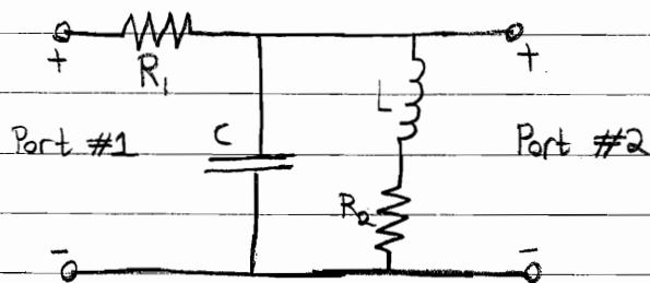
$$Z_{in,B} = R_1 + \frac{j\omega C (R_2 + j\omega L)}{R_2 + j\omega L + j\omega C}$$
