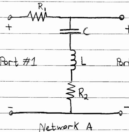
$$Z_{in,A} = R_1 + \frac{1}{j\omega C} + j\omega L + R_2$$
