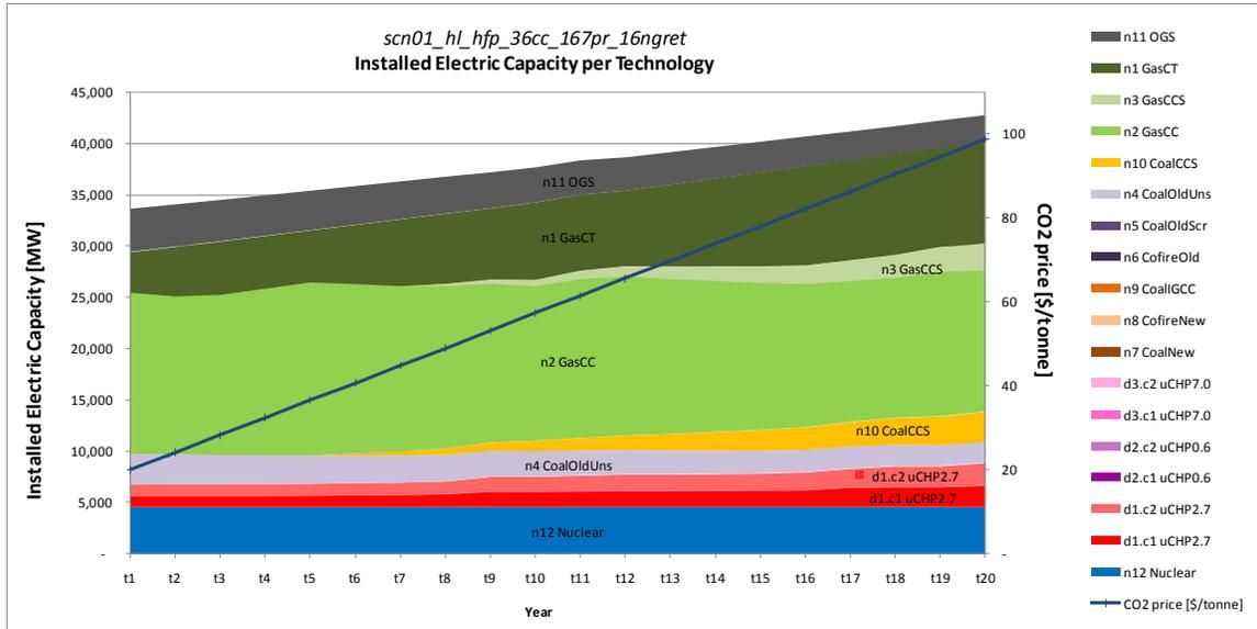
Figure 6.1.1: LT results for the case with micro-CHP - Electric installed capacity [MW] for every year of the time horizon for conventional generating and micro-CHP technologies
