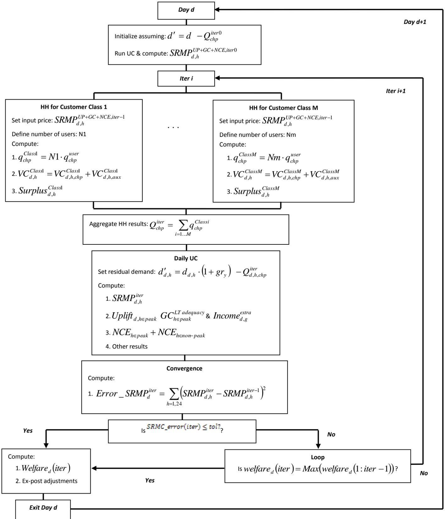
Figure 5.1.7: Short-term model complete iterative process
