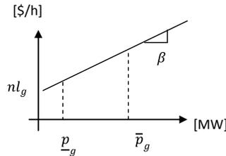
Where  $nl_g$  is the point where the generator ideally runs at zero power output (82),(110). This amount is paid to those units that are committed (on-line) to operate in the electric system.
