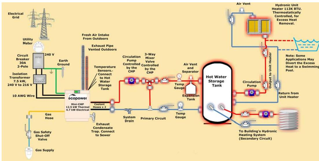
Figure 3. 1: Heating system with small-CHP
