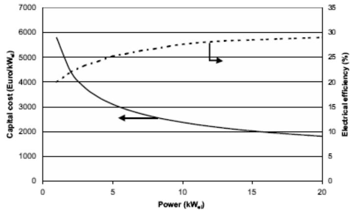
Figure 2.2.2: Capital cost & electrical efficiency for reciprocating engines
