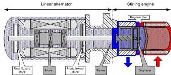
Figure 2.2.3: Free Piston Stirling Engine
