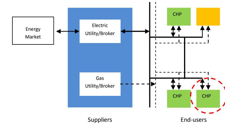
Figure 3. 2: Energy system representation with micro-CHPs
