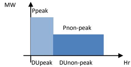
Figure 5.1.5: Two blocks electric load curve
