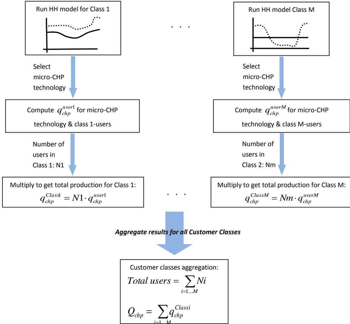
Figure 5.1.6: Methodology used for aggregating customers results
