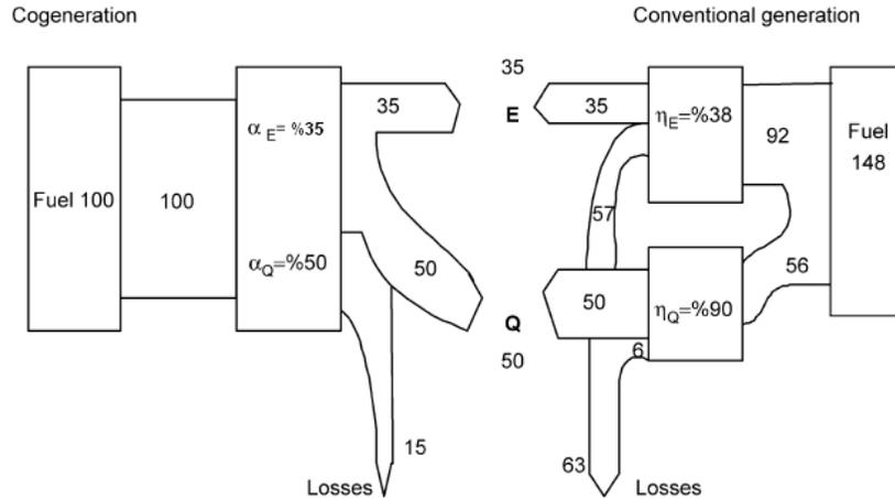
Fig. 1. Cogeneration versus conventional generation [4], where  $\alpha_E$ , part of the energy transformed into electricity in a cogeneration unit,  $\alpha_Q$ , part of the energy transformed into usable in a cogeneration unit,  $\eta_E$ , electrical yield of an electrical power plant (production of electricity only),  $\eta_Q$ , yield of a boiler (production of heat only),  $E$ , electricity demand,  $Q$ , heat demand.
