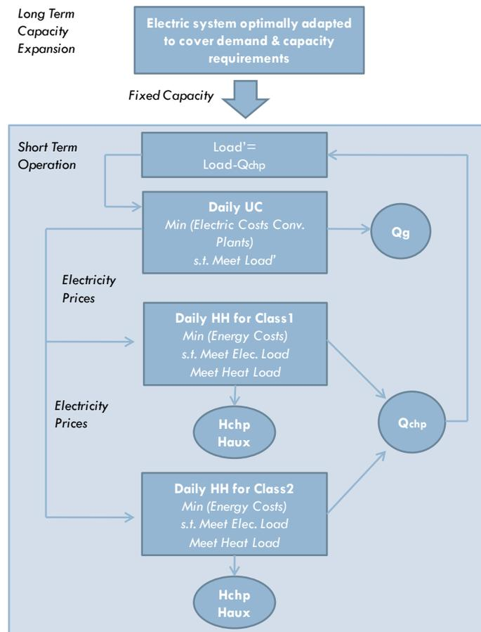
Figure 5.1.1: Short-term iterative process
