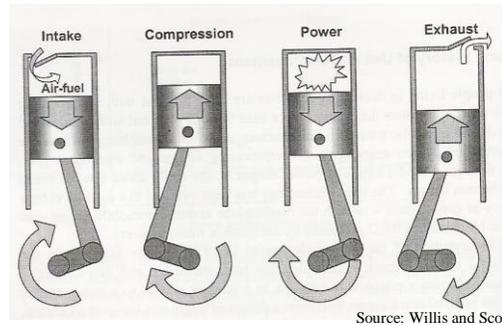
Figure 2.2.1: Otto cycle used in internal combustion engines
