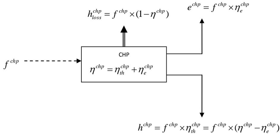
Figure A. 1 Micro-CHP energy outputs
