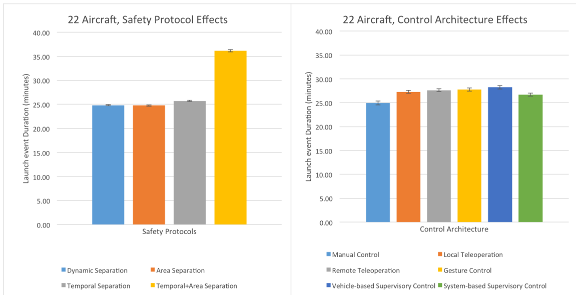
Figure 5-13: Column charts of effects of Safety Protocols (left) and Control Architectures (right) for 22 aircraft missions.
