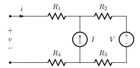
Exercise 3.3 (1 Point): Using the node method, develop a set of simultaneous equations for the network shown below that can be used to solve for the three unknown node voltages in the network. Express these equations in the form
