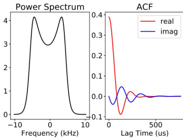
ISR theory gives the PSD and ACF of the received voltages as a function of  $N_e$ ,  $T_e$ ,  $T_i$ , and  $u_{\text{los}}$  in the overlap volume.
