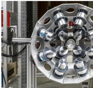
Atomki's new high-resolution \text{LaBr}_3 spectrometer, which will record gamma rays from excited nuclei. Credit: Atomki
