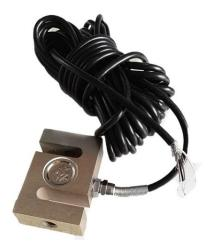
As for the test setup, each person on the sensing team will be constructing their own testing setup. The goal of each testing setup is to determine the best locations for the load cells on the exercise machine as well as determining how well the load cell measures forces for the
