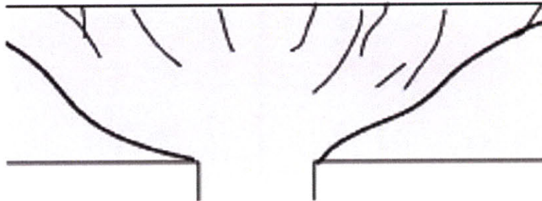
Figure 4-2: Punching Shear Failure (Tassinari)
