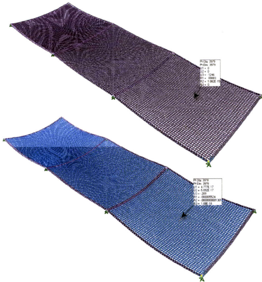
Figure 5-10: Maximum Bridge Deck Deflection Magnified by 100
