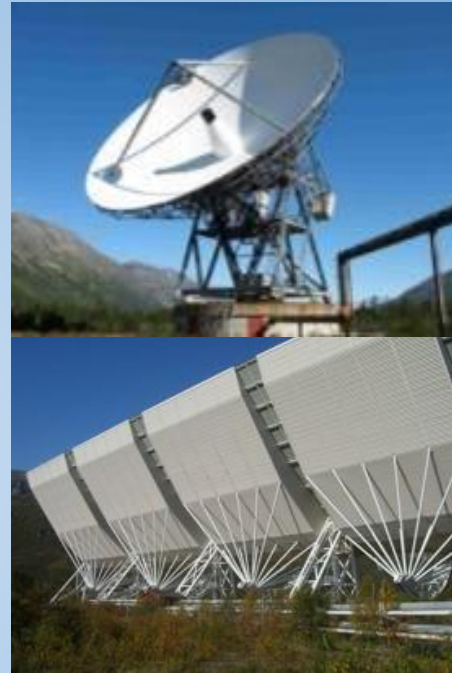
Photos of the UHF antenna (top) and VHF antenna (bottom). From the EISCAT Japan website.
