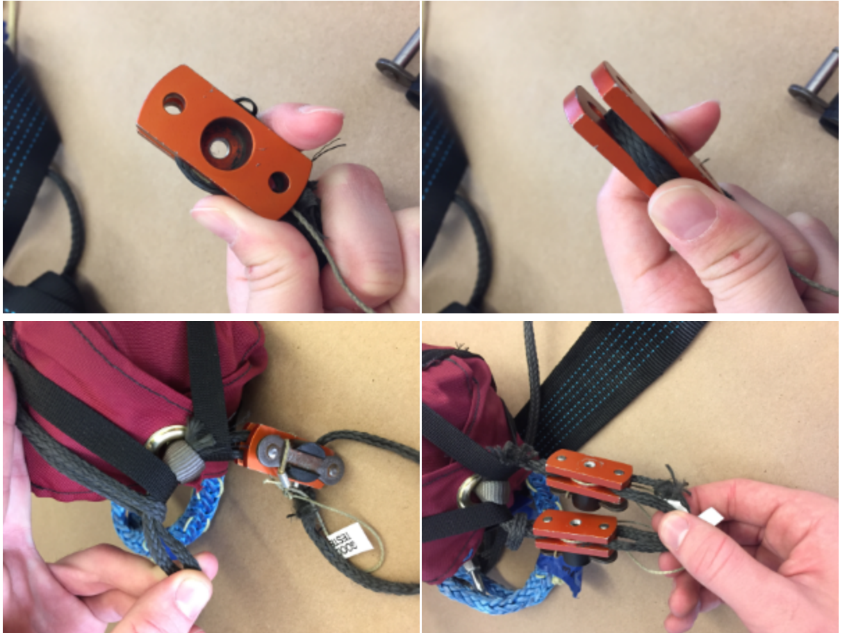
x. Connect white 1500lb swivel, TD loops, and TD restraining loops (thin yellow) to QL. Attach QL to eyebolt.
