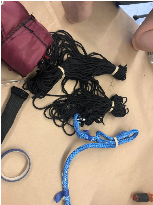
h. Pack lines into line-holding portion of the main bag and secure locking loop
