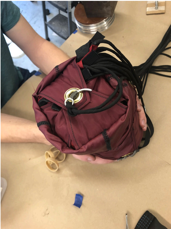
g. Fold lines into bites, secure two bites with rubber bands on both ends. Secure Main Riser (Spectra) in z-fold with 2 rubber bands.
