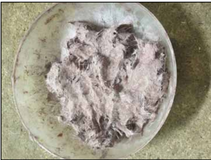
Photo 1: The slurry of ablative material before it was applied to the aluminum test sheet.
