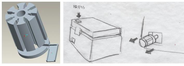
Vials are stacked in columns that can be rotated to dispense individual vials as needed. Different columns can store different vaccines, depending on the user's needs.
