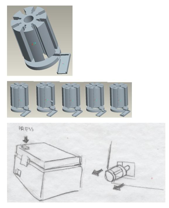
Vials are stacked in columns that can be rotated to dispense individual vials as needed. Different columns can store different vaccines, depending on the user's needs. The mechanism can dispense one vaccine vial at a time.
