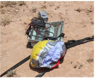
The payload did not deploy nominally due to shorted and deformed wires in the deployment electronics, and deformed parts in the motor housing for the CO2 deployment system.
