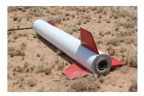
The avionics bay also largely withstood the landing, with a few broken pieces from the 3D printed adapters. The flight computers had some additional damage, and no data was taken from the Stratologger as a result. However, the flight computers with nylon pins fared better, as the nylon sheared, absorbing some impact energy. The motor case was unharmed.
