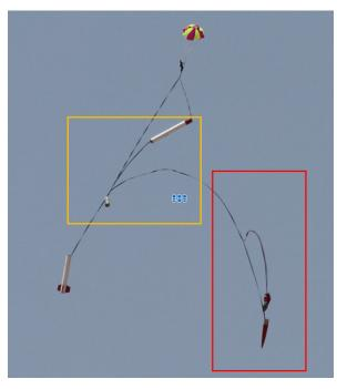
Here, a flaw in the recovery subsystem is revealed in the red box, and a tangling event between the payload (within the sabot) and the nose cone/main chute line in the yellow box.
