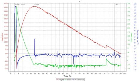
The Telemetrum data, combining GPS with barometric, is shown above. The jump in altitude near 112s is likely due to an updated GPS packet that affected the altimeters filter. It is unlikely due to a drop in pressure associated with the main chute being pulled out because the altitude was still above 1500 feet, the primary
