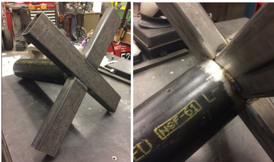
Welded Solid Test Stand Structure
