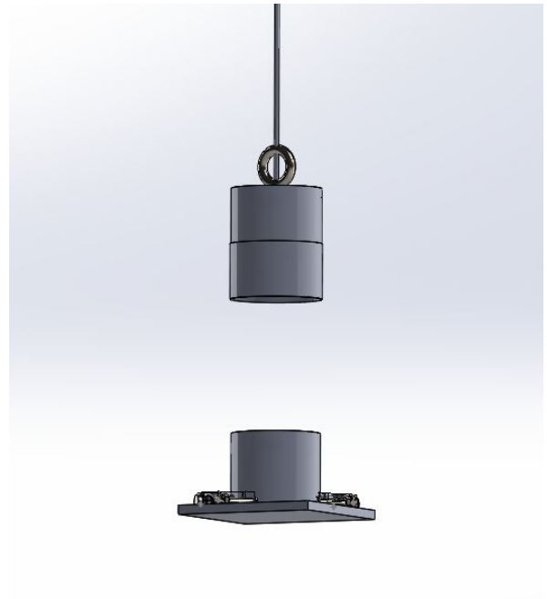
Released rover upon touchdown - spring assisted nichrome pin
