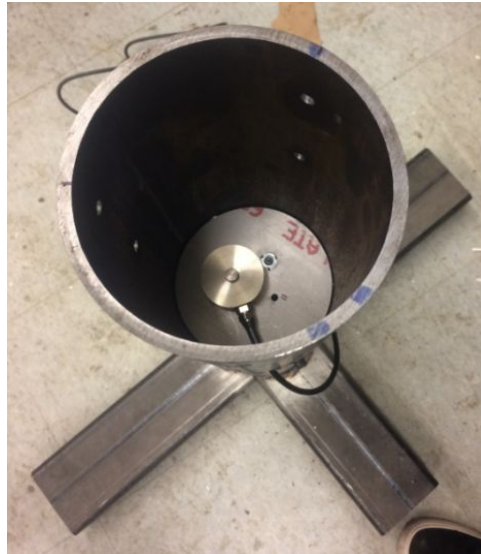
Solid Test Stand Mock Integration with Load Cell Mounting Plate and Load Cell
