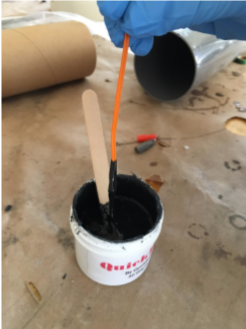
Manufacturing of the double-dipped igniters in the custom pyrogen mixture
