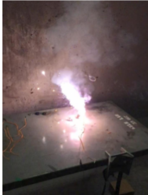
An igniter manufactured with the double-dipped method under test in the blast chamber.
