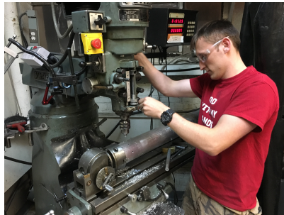
Kevin countersinks the radial bolt pattern on the case exterior
