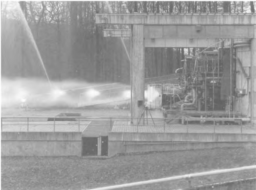
FIGURE 18–5. Visible plume created by the oxygen–hydrogen propellants of the Vulcain 60 thrust chamber, with a specific impulse of 439 sec at altitude, a nozzle expansion area ratio of 45, and a mixture ratio of 5.6. Multiple shockwave patterns are visible in the core of the plume because of emissions from luminescent minor species. (Courtesy of ESA/CNES/SEP/Daimler-Benz, Europe.)
