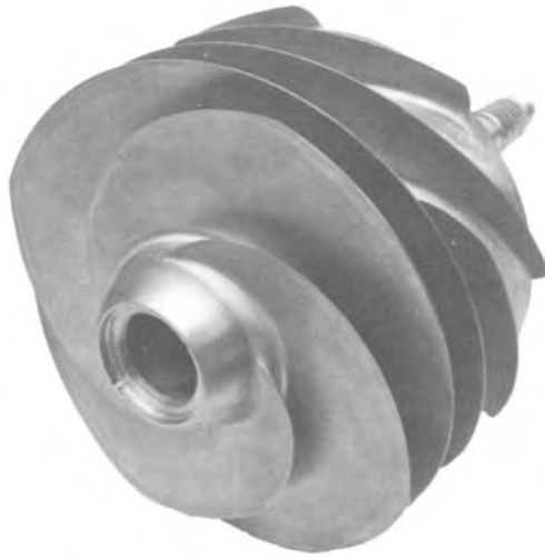
FIGURE 10-8. Fuel pump inducer impeller of the Space Shuttle main engine low-pressure fuel turbopump. It has a diameter about 10 in., a nominal hydrogen flow of 148.6 lbm/sec, a suction pressure of 30 psi, a discharge pressure of 280 psi at 15,765 rpm, an efficiency of 77%, and a suction specific speed of 39,000 when tested with water. (Courtesy of The Boeing Company, Rocketdyne Propulsion and Power.)
