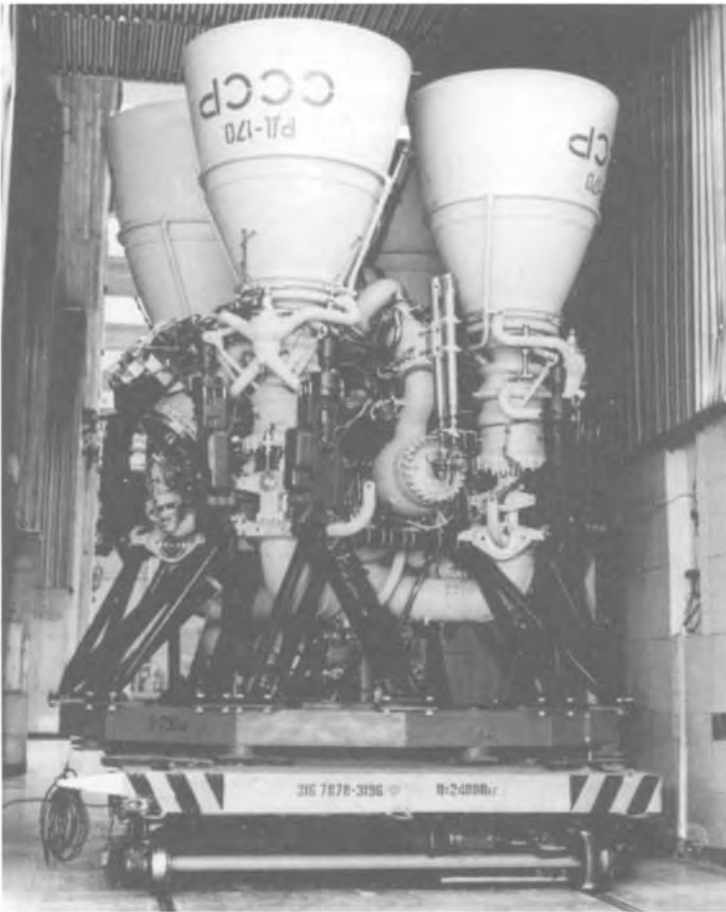
FIGURE 10–10. The RD-170 rocket engine, shown here on a transfer cart, can be used as an expendable or reusable engine (up to 10 flights). It has been used on the Zenith, Soyuz booster, and Energiya launch vehicles. The tubular structure supports the four hinged thrust chambers and its control actuators. It is the highest thrust liquid rocket engine in use today. (Courtesy of NPO Energomash, Moscow.)
