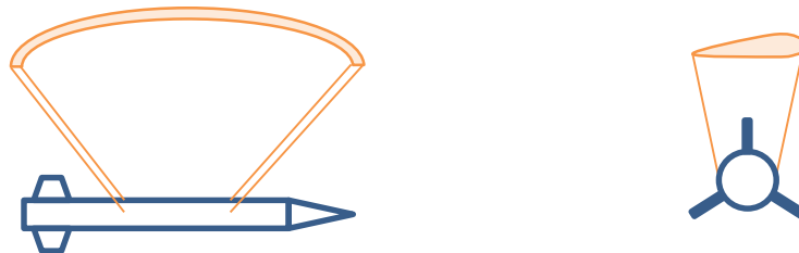
Figure 3: Side-first: Parafoil Oriented Parallel to the Axis of the Rocket
