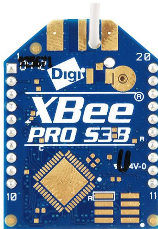
Figure 26: XBee Pro S3B Module with Wire Antenna (will be replaced with ducky via SMA) connector). (SparkFun, 2015)
