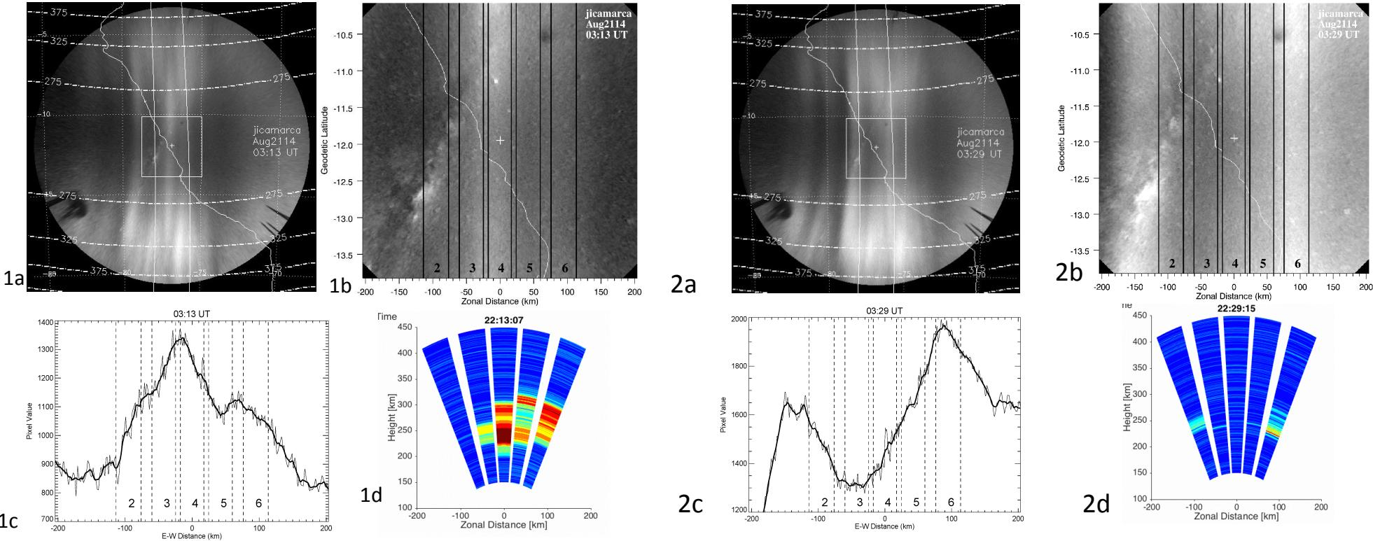
BU all-sky camera was installed at JRO in March 2014. The system can switch between 5 different filters (5577, 6300, 6950, 7774, 6050A). ESF observations taken with this system and AMISR (Aug 2014) are compared to study the relationship between air-glow structures and coherent scatter radar echoes.
