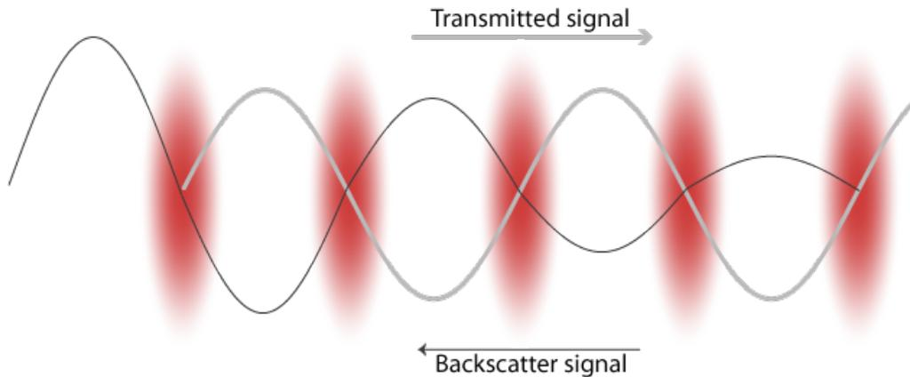
Backscatter is amplified under Bragg conditions by density fluctuations with scale sizes on the order of half the transmitted wavelength.
