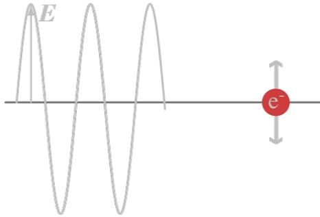
EM backscatter generated by free electrons in the ionosphere accelerated by a transmitted signal.
