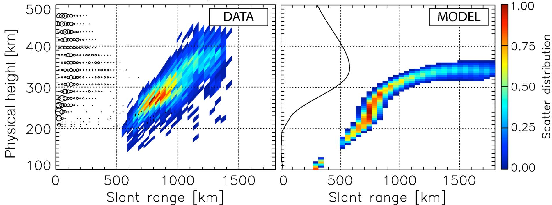
Altitude versus slant range plots of quiet –time subauroral backscatter from SuperDARN (color) and of electron densities from MHO (bubbles) and from the IRI model (line). As suggested by the comparison to the model, the observations with MHO indicate that the irregularities occur mostly below the F-region peak.
