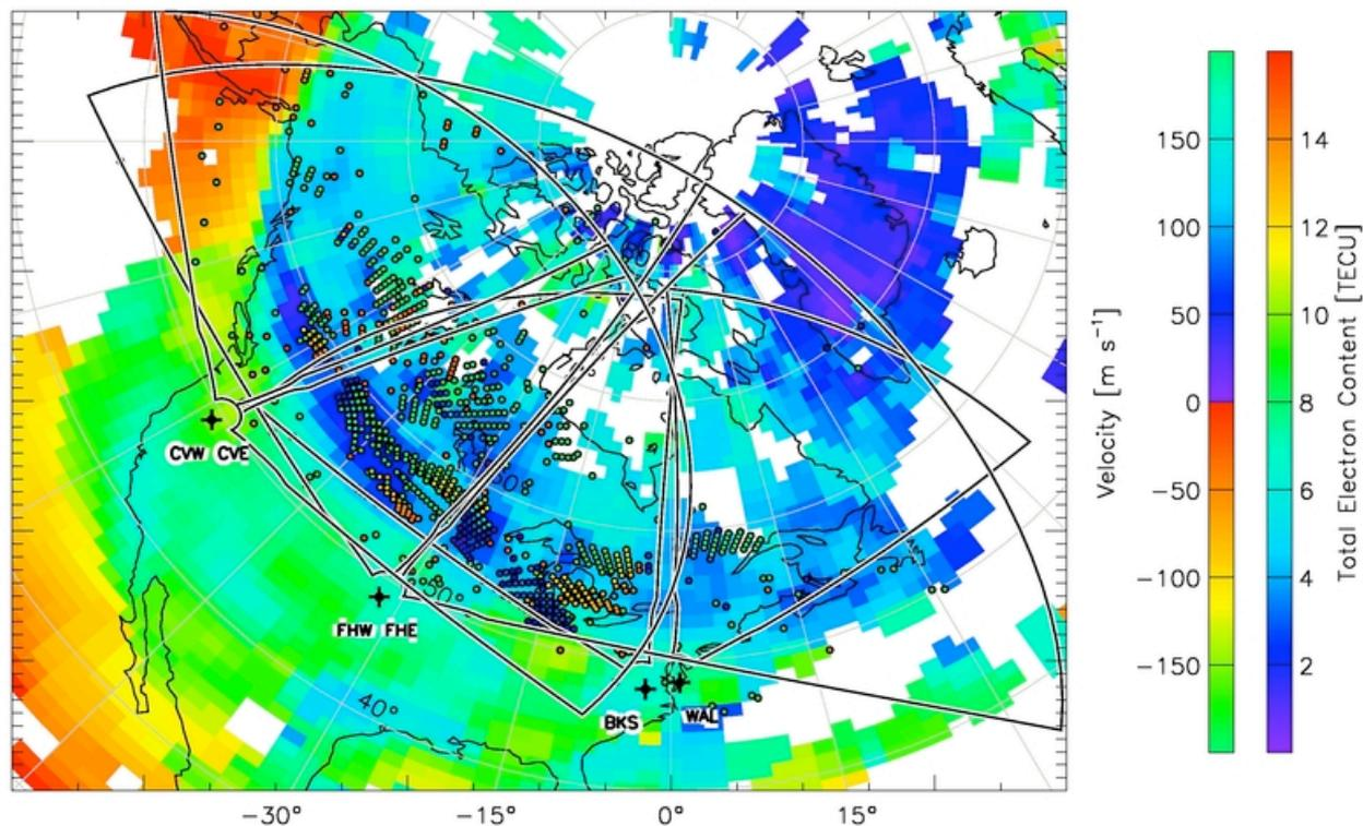
Plot of SuperDARN backscatter velocity measurements overlaid on median filtered TEC values for March 11<sup>th</sup>, 2011.
