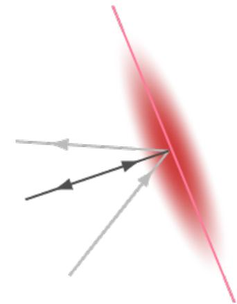
Orthogonality of the transmitted signal with the background magnetic field (aspect condition) guarantees maximum returned power.
