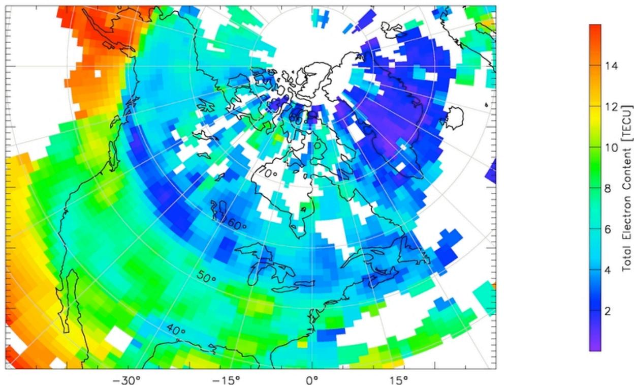
Plot of median filtered TEC values over North America for March 11<sup>th</sup>, 2011 created on the GPS/TEC Plot page of the VT website.
