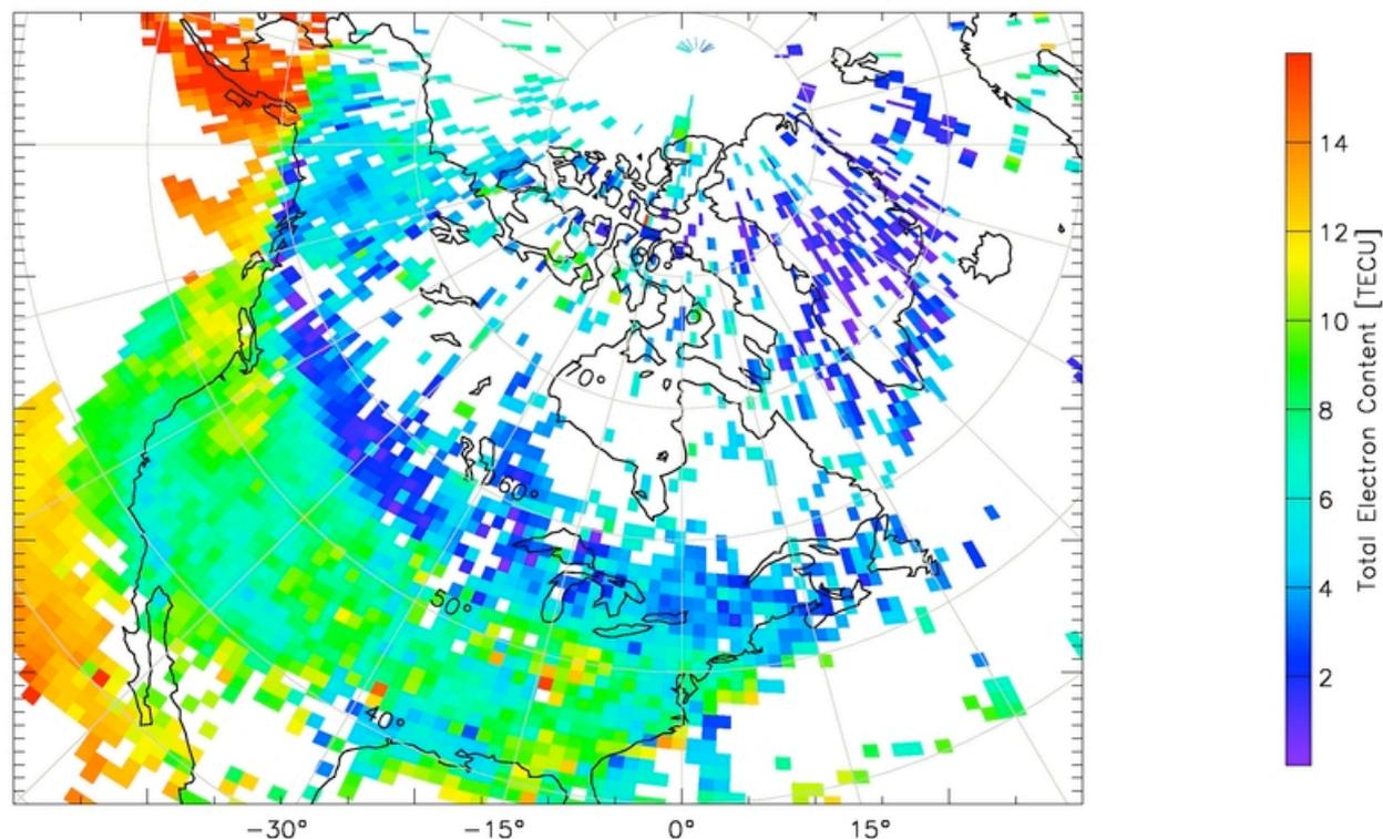
Plot of unfiltered TEC values over North America for March 11<sup>th</sup>, 2011 created on the GPS/TEC Plot page of the VT website.
