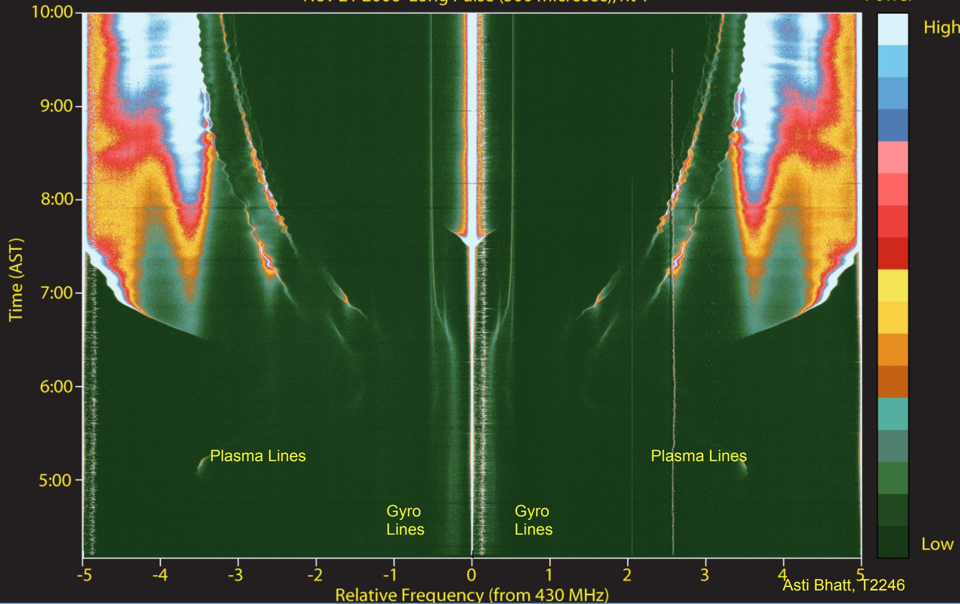
Arecibo Sensitivity: The 305 m dish, 2.5 MW of power, and  $T_{\text{sys}}$  of about 80 K (condition dependent) provide high time resolution on even weak features such as the gyro line. The data above are centered on the E region. The strong plasma line after sunrise is “leakage” from the low F region. The complicated behavior of the gyro line is probably due to multiple layers, but is not completely understood.
